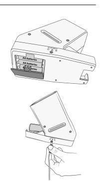
Once the slide viewer is connected to a power source (either battery or adapter), firmly press and release the power button. The power button is located on the bottom right side of the slide viewer, opposite the adapter port. The light will turn on and stay on, confirming the device is powered. To turn the light off, press the power button again.
