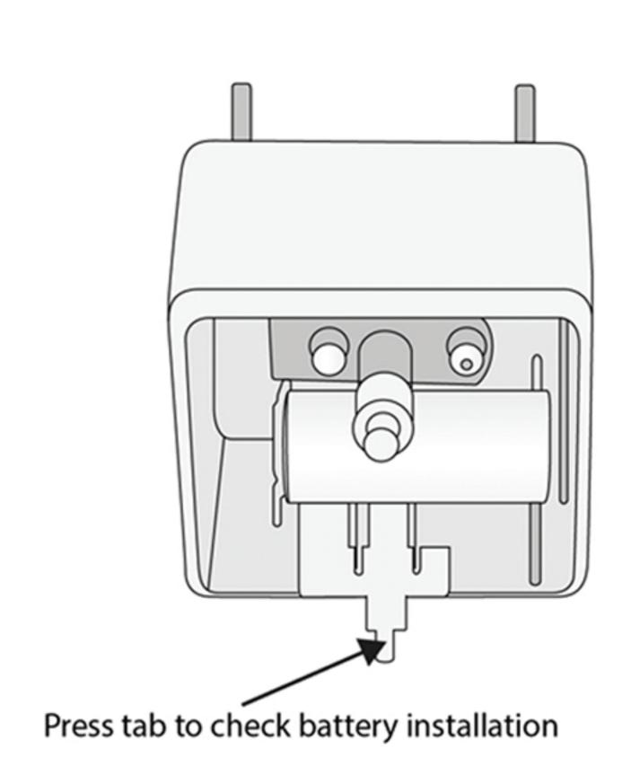
Once the batteries are installed, lightly press down on the protruding metal tab. The light bulb should turn on, confirming the batteries are installed correctly.
